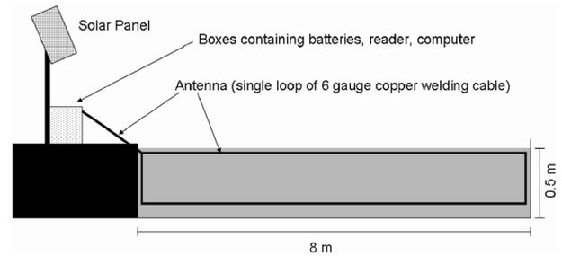
Fig. 2. Schematic of the antenna system shown in a creek cross-section view. The dimensions of the antenna loop are the same as the creek, but the antenna is shown slightly smaller than the creek dimensions for clarity.
